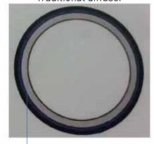
small airgap makes airflow difficult and increases head los
